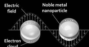
Combining fluorophores into a concentric nano-architecture can lead to **metal-enhanced fluorescence (MEF)**, allowing a better sensitivity for detection.<sup>4</sup>
